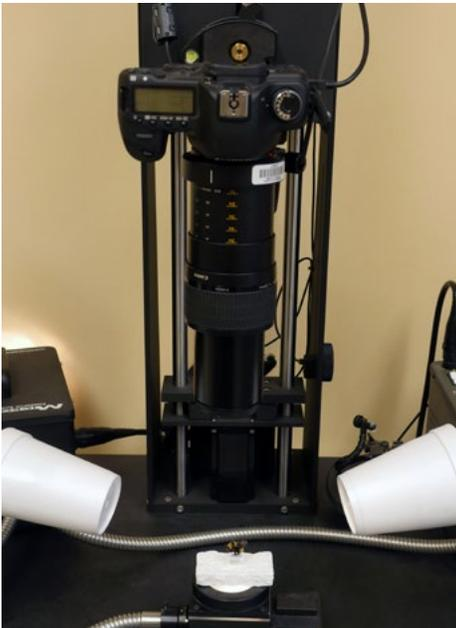
ABOVE: Camera set up to photograph insects
