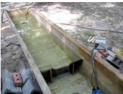
*A simulated spillway. Photo by Max Wolter, INHS*
