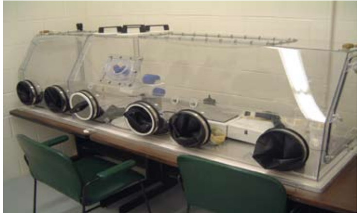
Glove box used to separate blood-fed from unfed female mosquitoes and to dissect blood-fed mosquitoes that survive the 14-day virus incubation period. Photo by Ephantus Muturi
